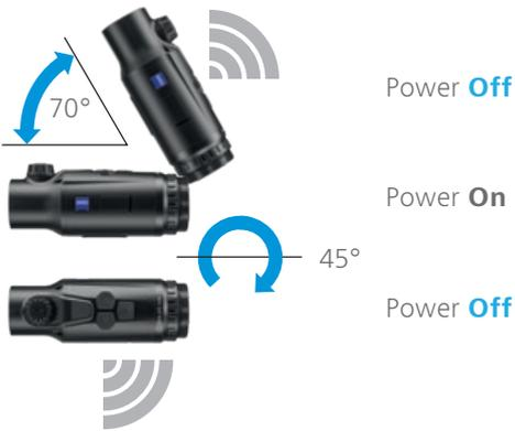
The angle sensor automatically detects the exact position of the ZEISS DTC 3 and activates standby mode at a lateral angle of 45° and at a downward or upward angle of 70°. When the hunter brings the weapon back to the firing position, the device automatically exits standby mode.
