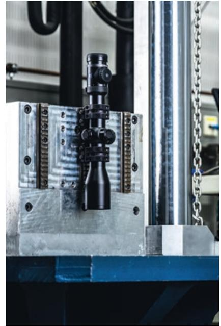
**Testing extreme situations:** significant temperature fluctuations within minutes and shot simulations with 1,500 times the force of gravity.
