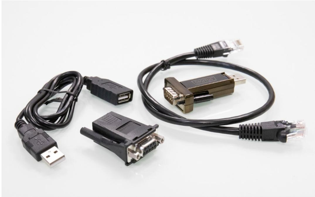
While the RJ45 "PC" port on the EFA is similar to that used for Ethernet, the protocol used for communication with the PC is serial/RS232 and the wiring differs from that of Ethernet. The included USB-to-serial adapter, USB extension cable, DE9-to-RJ45 and standard CAT5 cable must be used rather than a direct connection via Ethernet to the PC. If needed, a longer CAT5 cable can be used to extend the connection between the DE9-to-RJ45 adapter at the PC and the EFA.
