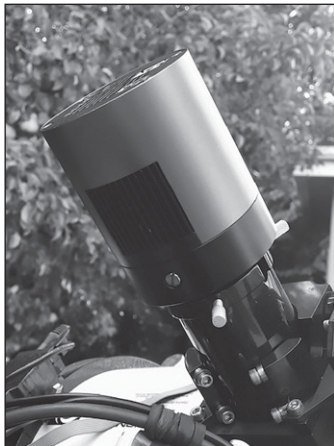
Figure 3a. The G10, installed in a 2" focuser using the included 2" nozzle
