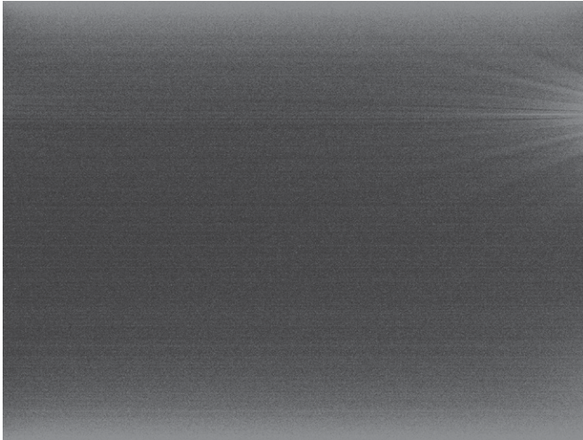
Figure 10. A 120 second dark frame. Note the amp glow on the upper right side, this is standard for the ICX294 chip, and is removed from light images during dark frame subtraction.
