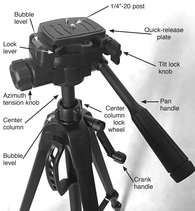
Figure 2. Features of the Tritech LT-1 pan head.
