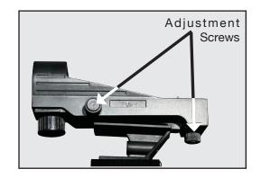
Now, without moving the telescope, adjust the indicated thumb screws until you have put the red dot on the object at which you were looking. It's that simple.
