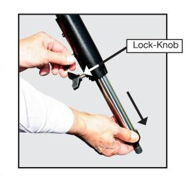
**3** Thread in the lock-knobs on each leg near the foot of each tripod leg. Use the lock-knobs to vary the height of the inner, extendible tripod leg sections. Tighten the locks to a firm feel only; do not overtighten.
