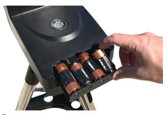
**6** Remove the end cover from the battery compartment exposing the battery tray. Carefully slide the battery tray out until it reaches its end stop. Insert 8 (user supplied) Alkaline "C" batteries into the battery compartment. Take care that the batteries + and - ends are as indicated in the battery holder.
