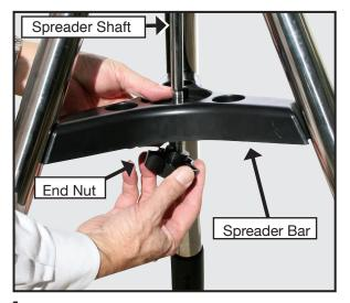
**4** Remove the end nut from the spreader shaft and slide the spreader in between the telescope legs. Attach the end nut and hand tighten until the telescope legs are held snuggly in the most spread position. Position the tripod where you want the telescope to be and check that the top of the tripod is approximately level.
