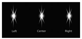
**Figure 5.** As the telescope's focus is adjusted, the middle spike of the diffraction pattern moves left and right of center of the "X" formed by the other two diffraction spikes. Adjust focus until the middle spike is exactly centered in the X; that's when precise focus has been achieved.
