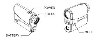
The GX-5i<sup>3</sup> has two buttons: POWER and MODE. When you initially press the POWER button, the display is activated and the unit is ready for ranging. Press the POWER button a second time to range, or hold the POWER button depressed to scan. Scanning automatically updates the display. When ranging without a steady rest at long distances, you can easily differentiate the pin from other potential targets behind the pin.
