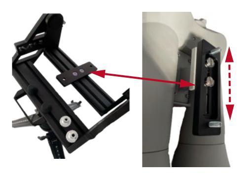
In order to mount the binoculars on the fork mount, the rail must first be screwed onto the binoculars. To do this, use the two screws as shown in the lower picture. Depending on the size and weight of the binoculars, the weight balance can be set variably by moving the mounting rail on the bottom side of the binoculars.
