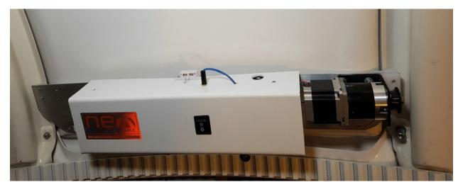
Feed-in the track under the motor sprocket by using the direction rocker switch. Feed the track for 4-5 inches.
