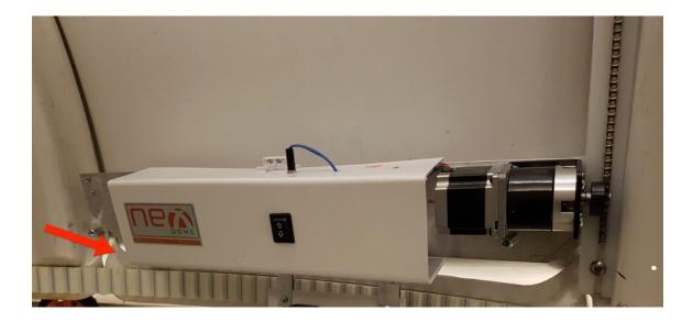
Move the shutter to fully open position and attach the magnetic the **"Open"** magnetic limit sensor in front of the shutter magnet on the edge of the dome back panel.
