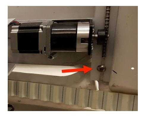
Fasten the track to the coupler with the provided screw on the track end.
