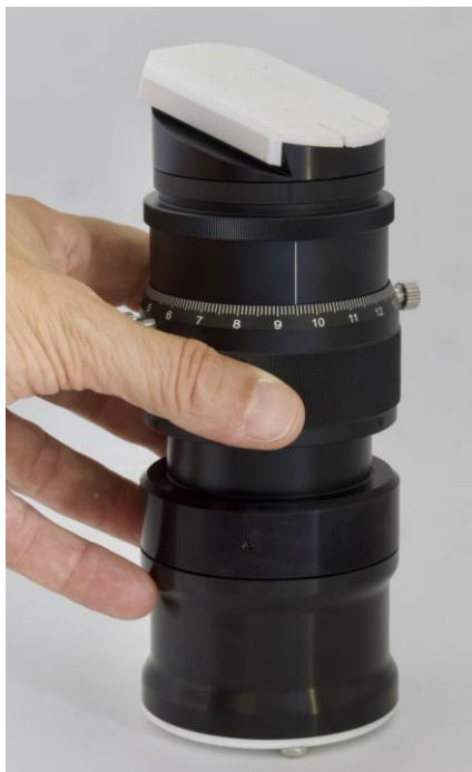
Custom-calculated 122 mm Petzval lens. The lens focusing ring is noticeably smoother than on the eShel II
