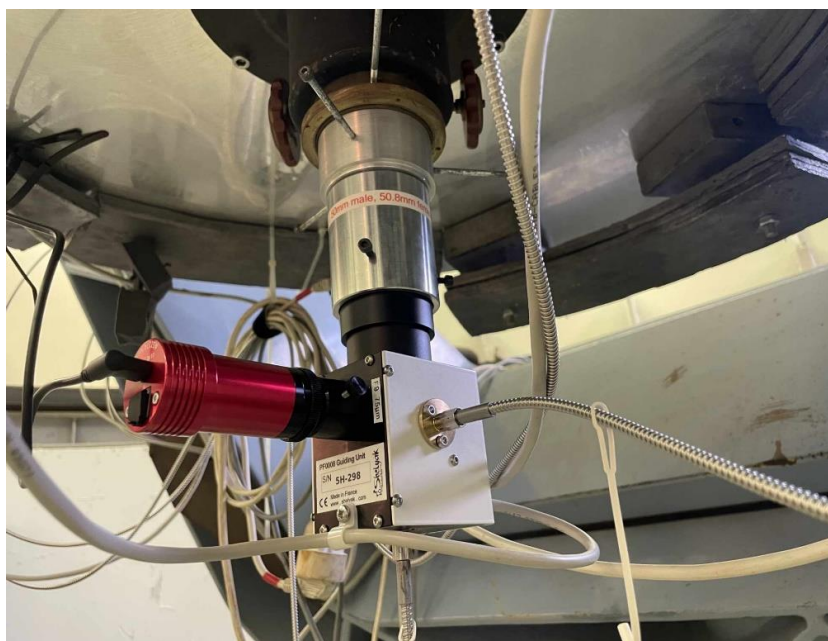
The head installed at the telescope focus, with its autoguiding camera and the two optical fibres — Photo credit: Olivier Garde
