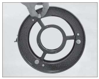
**Figure 23.** The three small thumbscrews that lock the primary mirror in place must first be loosened before any adjustments can be made. Then the tilt of the primary mirror can be adjusted by turning one or more of the three larger thumbscrews.
