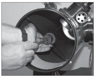
**Figure 21.** To center the secondary mirror under the focuser, hold the mirror holder in place with one hand while adjusting the center bolt with a Phillips screwdriver. Do not touch the mirror's surface!
