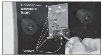
Figure 6. Attaching the encoder connector board.
