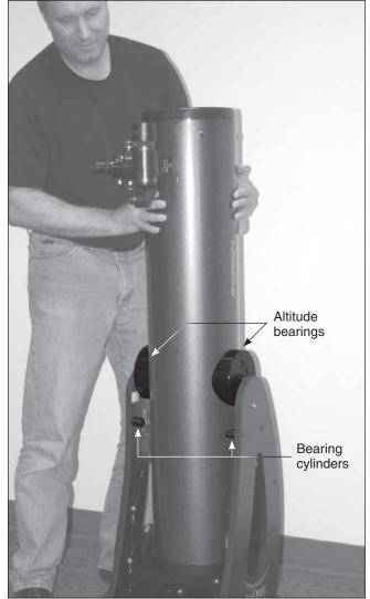
**Figure 9.** Lift the optical tube and place it into the Dobsonian base so that the altitude bearings rest on the bearing cylinders. Orient the optical tube as shown. Do not bump the encoder connector board or vertical stop when installing the optical tube.
