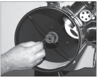
**Figure 22.** Adjust the tilt of the secondary mirror by loosening or tightening the three alignment set screws with the 2mm hex key.
