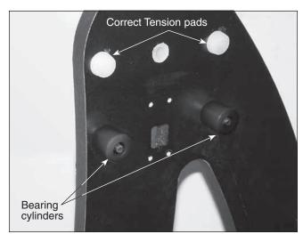
Figure 5. Attaching the bearing cylinders.
