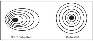
**Figure 24.** A star test will determine if a telescope's optics are properly collimated. An unfocused view of a bright star through the eyepiece should appear as illustrated on the right if the optics are perfectly collimated. If the circle is unsymmetrical, as in the illustration on the left, the scope needs collimation.
