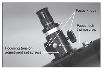
Figure 13b. The 1.25" rack-and-pinion focuser of the SkyQuest
