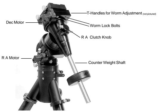
\*The Titan is shipped with its Latitude set at 20-42 degrees. For other degrees, loosen altitude lock, remove six bolts through the access holes (3 per side), move head in the desired direction until next available hole pattern aligns, re-insert six bolts.
