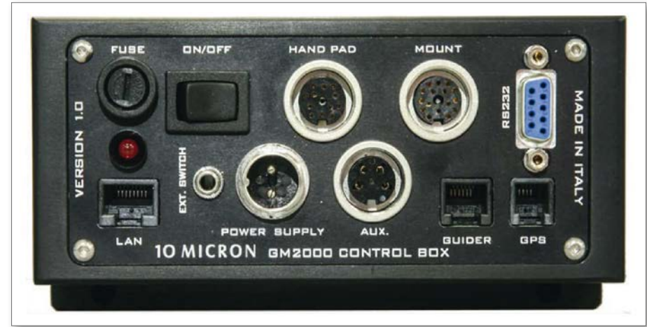
The connections of the control box
