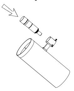
Remove the dust cover and Loosen the thumbscrews on the end of the focuser adapter.
