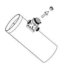
Insert the 1.25" or 2" eyepiece and lightly tighten the thumbscrews to hold the eyepiece in place.
